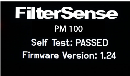
Step5 - Power Up Screen Showing "Self-Test: PASSED"
