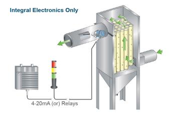
As particles flow over a sensing probe, charge is induced into the probe creating small currents in the picoamp (pA) range. The signal is processed into an output proportional to mass.
