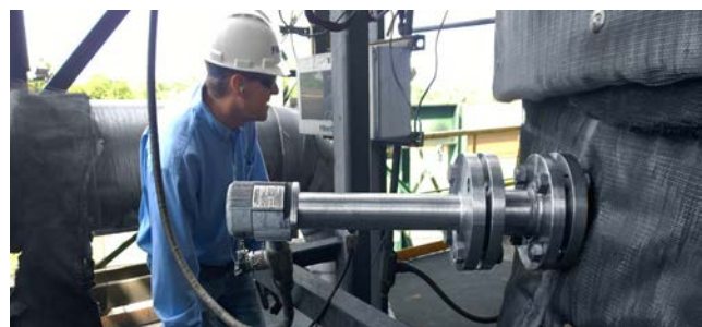
A PS 10 sensor is installed providing reliable performance in the outlet of a dryer drum; Auburn engineer observing control unit display.
